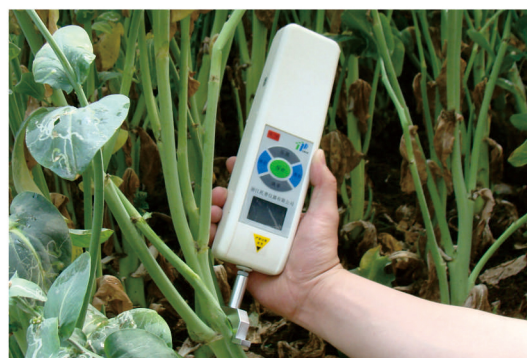
two different fixtures for measuring the strength of different crops
