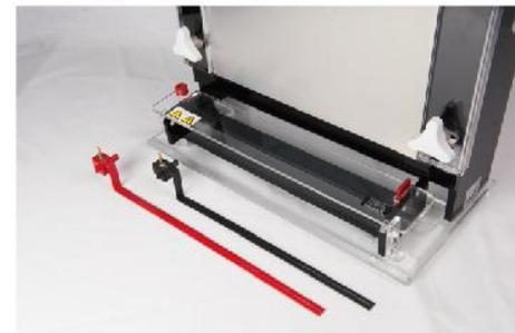
● Unfolded electrodes
