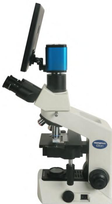
Side View of Olympus Microscope+XCAMSeries Camera and TPHD1080PA
