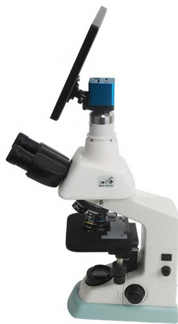
Side View of Nikon Microscope+XCAMSeries Camera and TPHD1080PA
