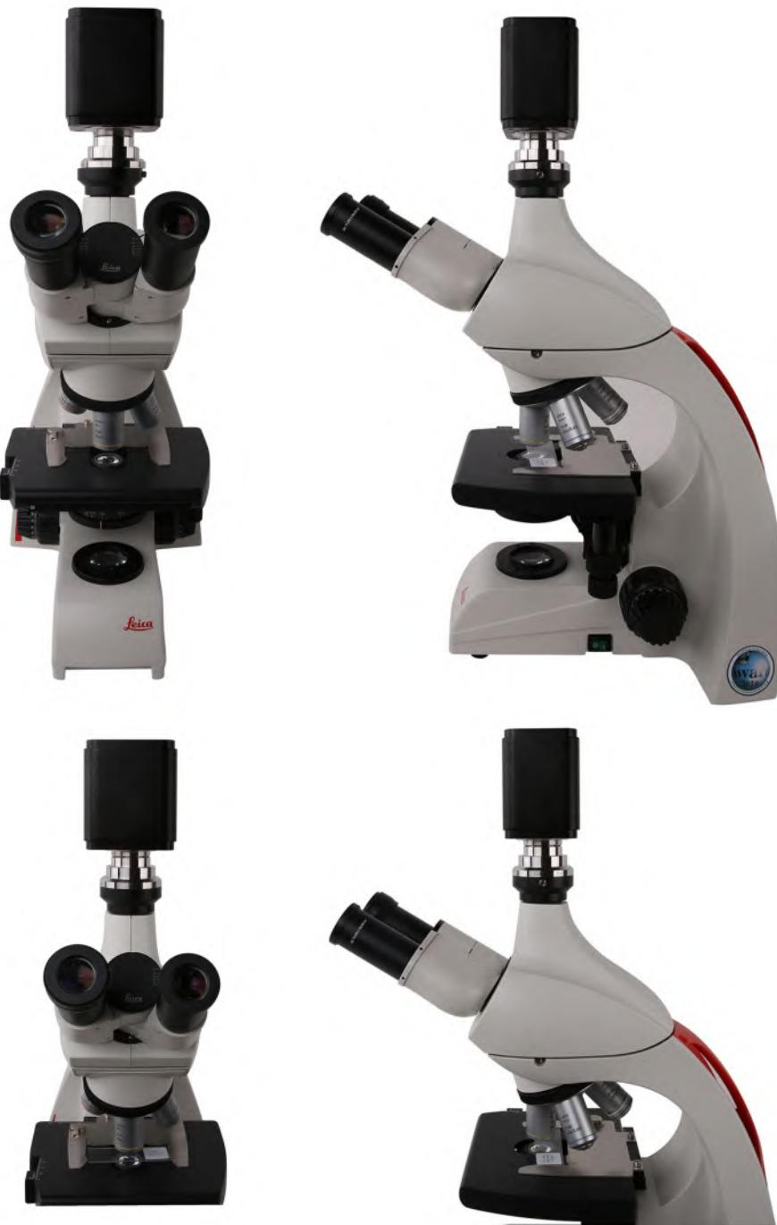
Figure 5-1 XCAM4K Camera and Leica Microscope
