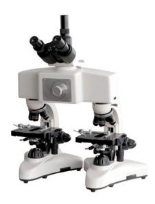
Model XZB-605 Comparison Microscope makes you view two images (left & right) from two objects at the same time. Adjusting two images to connect or lap over, then differentiate the minuteness difference between them, for instance, identifying the bullet's mark, tool's mark, fingerprint, stamp, letters, money, presswork, etc. It is an ideal instrument for Police and other departments, which need object comparison.
