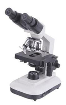
Achromatic objective: 4X,10X,40X(S),100X(S,OIL) Eyepiece: WF 10X Eyepiece head: Hinged Binocular Head Nosepiece: Quadruple Stage: Double Layer Mechanical Stage Size 125X115mm Focusing: Coaxial Coarse and Fine Adjustment, Focusing Range 20mm, Focusing Interval 0.002mm. Condenser: Abbe NA=1.25 with Iris Diaphragm &Filter Illumination: 6V/20W Halogen Lamp
