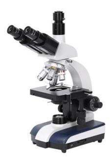
Achromatic objective: 4X,10X,40X(S),100X(S,OIL) Eyepiece: WF 10X/18mm Eyepiece head: Hinged Trinocular Head Nosepiece: Quadruple Stage: Double Layer Mechanical Stage Size 130X125mm Focusing: Coaxial Coarse and Fine Adjustment, Focusing Range 30mm, Focusing Interval 0.002mm. Condenser: Abbe NA=1.25 with Iris Diaphragm &Filter Illumination: 6V/20W Halogen Lamp
