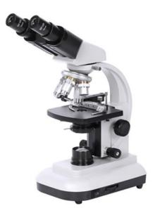
Achromatic objective: 4X,10X,40X(S),100X(S,OIL) Eyepiece: WF 10X/18mm Eyepiece head: Hinged Binocular Head Nosepiece: Quadruple Stage: Single stage with moving scale Focusing: Coaxial Coarse and Fine Adjustment, Focusing Range 30mm, Focusing Interval 0.002mm. Condenser: Abbe NA=1.25 with Iris Diaphragm &Filter Illumination: 6V/20W Halogen Lamp
