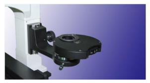
Reflected fluorescence Illumination System Pushed fluorescence filter provides four fluorescence filter system shuc as UV, V, B and G. This kind of frame can make it switch fleetly between each fluorescence system. 100W mercury lamp can provide ample illumination for fluorescence observation. Equip power supply unit.
