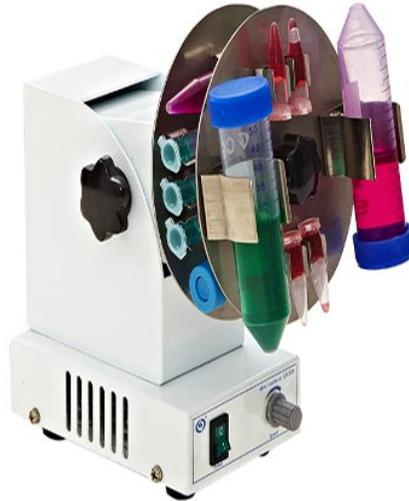
Adjustable rotational Angle, horizontal position for slightly mix, vertical position to fully mix.
