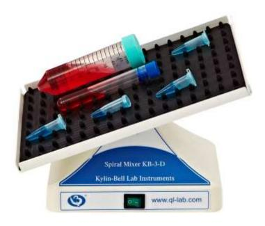
This is a small mixer that can be used in the cold storage house. It is suitable for mixing of blood collection. The mixing movement of this mixer is three-dimensional and does not produce bubbles. It is the ideal choice for a sample with a small dose. The concave pad of the KB-3-D mixer can firmly fix tubes. Applicable tubes are  $60 \times 1.5 \text{ml}$ ,  $30 \times 3 \text{ ml}$ ,  $21 \times 7 \text{ ml}$  and  $17 \times 15 \text{ ml}$ .
