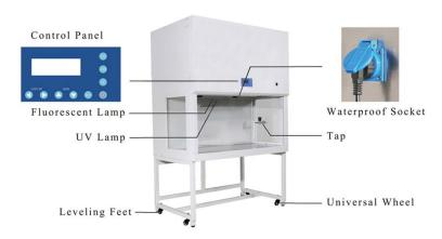
Laminar Flow Cabinet is a work bench or similar enclosure, which creates a particle-free working environment by taking air through a filtration system and exhausting it across a work surface in a laminar or unidirectional air stream. The laminar flow cabinet is enclosed on the sides and kept under constant positive pressure in order to prevent the infiltration of contaminated room air.
