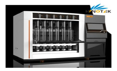
F800 Fiber Analyzer is with advanced design, easy operation and flexible application. It can be used in conventional Weende method to analyze crude fiber and Van Soest analysis to wash the fiber. Applies to plant, feed, food and other agricultural products as well as the determination crude fiber, neutral detergent fiber (NDF), acid detergent fiber (ADF), hemicellulose and acid detergent lignin (ADL).
