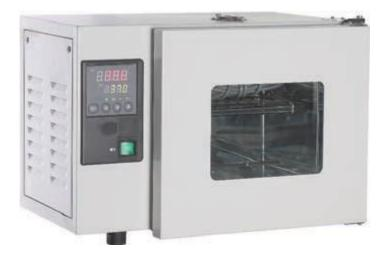
Microprocessor controller (with timing function)
