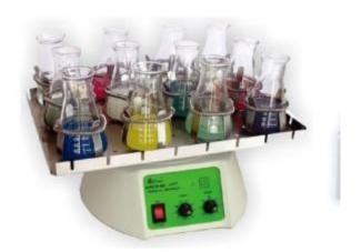
"Start" or "Stop" operation can be controlled by front panel function keys or "Start" controlled by connection key while the "Stop" operation controlled by timer flat forms function.
