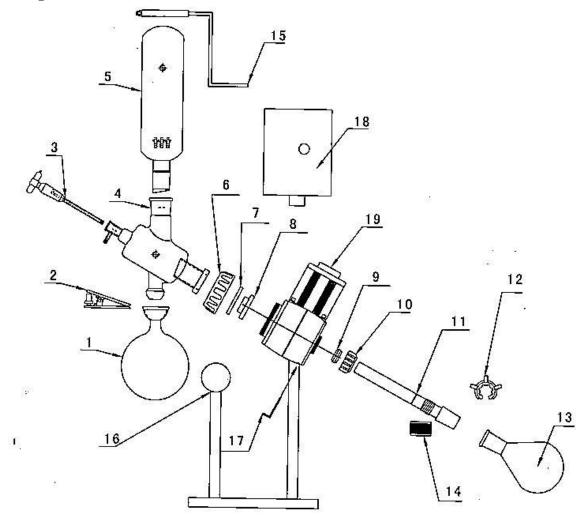
1. Receiving Flask 2. Clamp for Receiving Flask 3. Inlet Valve with Stop Cock 4. Distribution Piece 5. Vertical Condenser 6. Big Nut 7. Gasket 8. Seal 9. Cramp Ring 10. Small Nut 11. Vapor Duct 12. Clip for Evaporating Flask 13. Evaporating Flask 14. Flask Unloader 15. Support Rod Complete 16. Vacuum Meter 17. Brake Bar 18. Rotary Speed Controller 19. Motor
