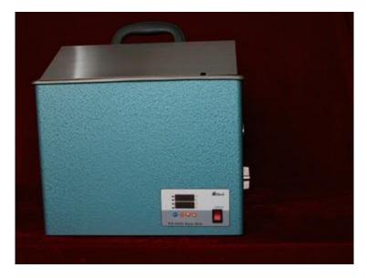
**Micro programmable PID controller** reduces the temperature difference inside shaking bath and smoothly rises the temperature.
