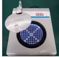
Have the function of counting in bidirectional Caxial lighting, 3 times enlargement, 9 times enlargement.
