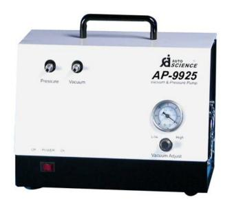
Type:AP-9925Max vacuum (Kpa):0-80 AdjustableMax Pressure(psi):20Free-air Capability (l/min):25Power (VA):120Power supply:AC220V/50HzDimension (mm) :269Lx210Wx155HShpg (Kg) :7.3 Advantage
