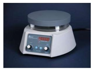
The products working theory uses micro-electrical charges driving the heatproof magnet to spin in order to create a magnetic field. This magnetic field will drive the stir bar to spin in the container to achieve the purpose of spin for the solvent. Meanwhile, it can heat the solvent to it them fully mixed and reacted at the set temperature. This product is widely applied to biology, medicine, chemistry, chemical engineering and other fields
