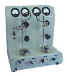
This instrument is a complete set of equipment for the analysis of nonferrous metal by electrolysis. The suitable electrolytic solution and current intensity or breakdown voltage can be used to analyze the elements such as copper, lead, nickel, tin and zinc, and achieve the purpose of quantitative analysis.
